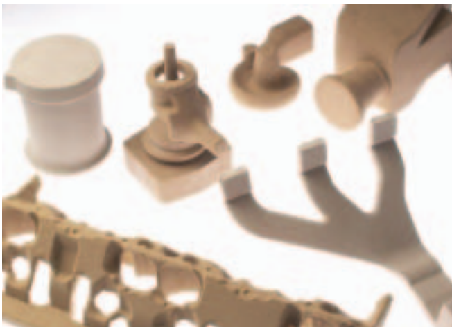
Cores formed with environmentally friendly sand binders offer performance similar to cores made with petroleum-based binders.
